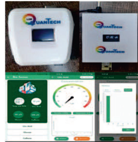
Fig. IoT-enabled portable uric acid sensor system integrated with android/iOS mobile application for real-time monitoring.
