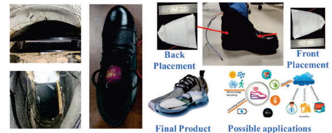
Fig: TENG integrated shoe sole for powering wearable electronics
