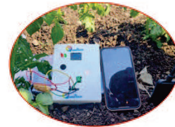
Fig. Developed IoT-enabled portable soil health monitoring system (Bhu-Samvardhak).
