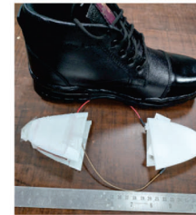
Position of TENG inside the sole
